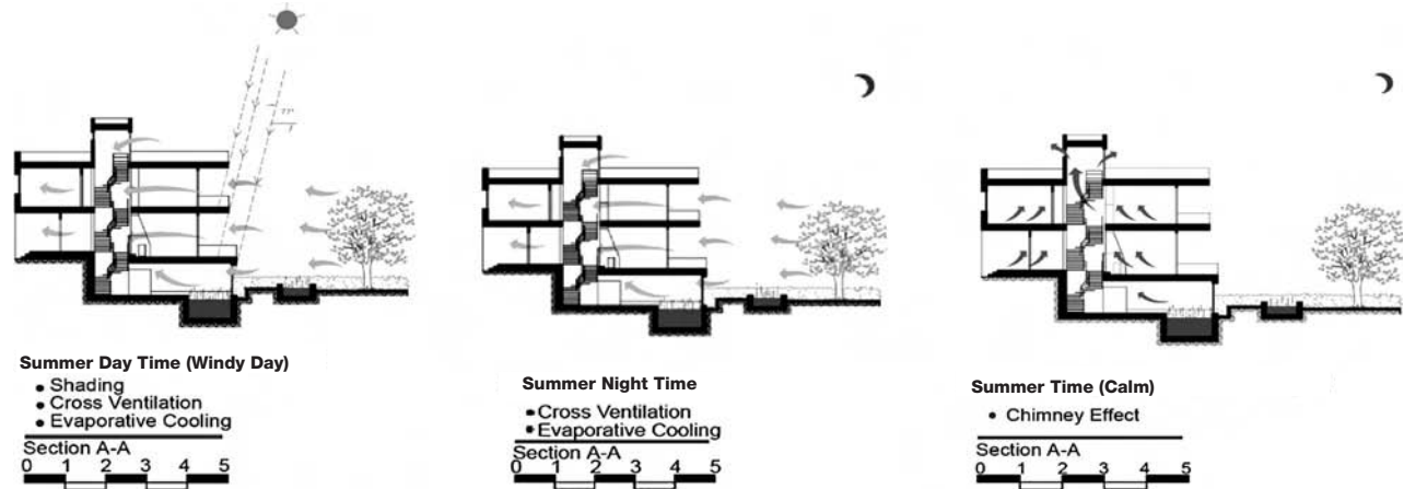
5.7 Summer thermal strategies for the row house in Figure 5.6, as seen through section A-A
